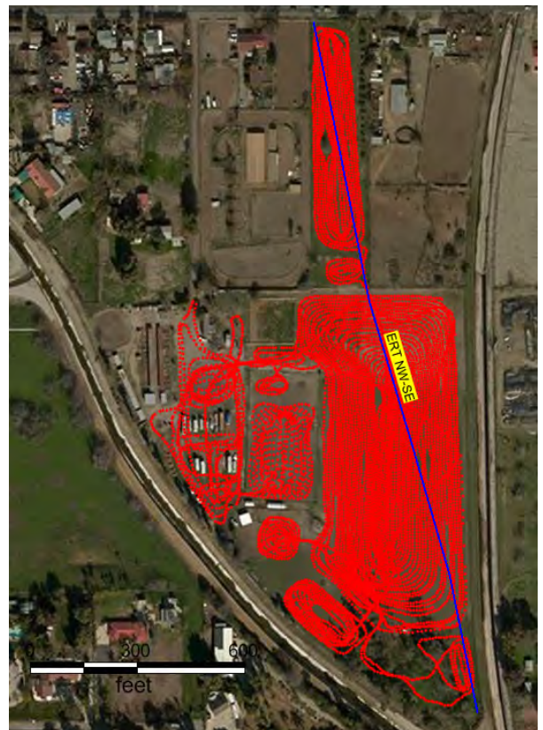
Figure 10: DUALEM data marked with red and the collected ERT marked with blue.
