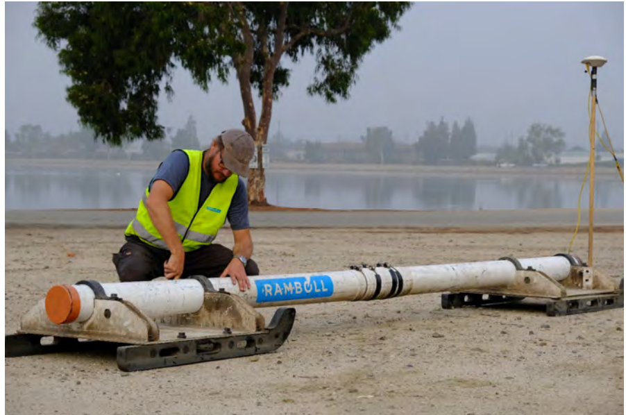
Figure 4: Assembling the DUALEM system
