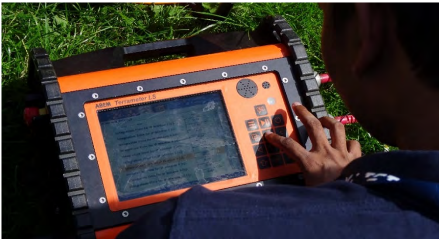
Figure A2-2: The LS-Terrameter in operation
