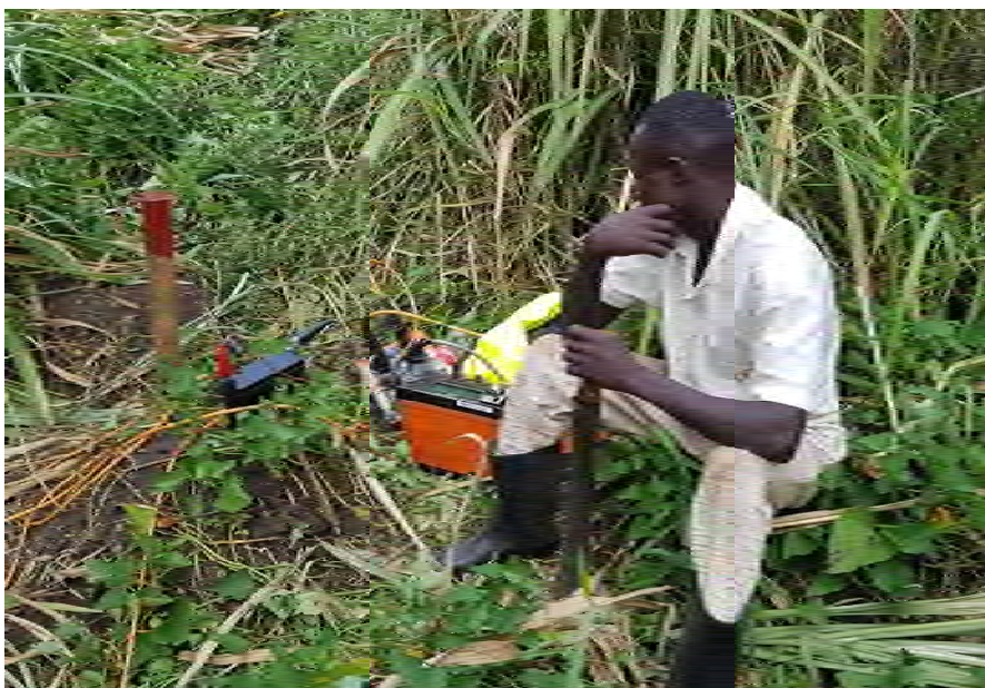
Figure A2-4: The SAS4000 Terrameter and ES-10-64C switch box in operation
